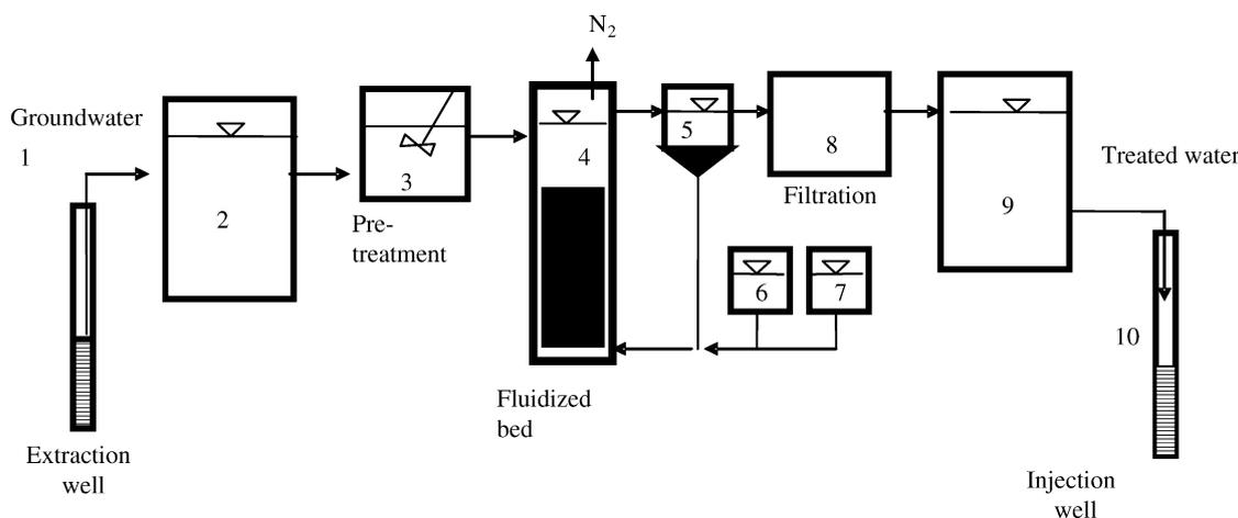
**Fig. 1** Schematic diagram of fluidized bed reactor system for removal of nitrate from contaminated groundwater. 1 indicates extraction well; 2, groundwater storage tank; 3, pretreatment units (VOC removal, pH adjustment, and dissolved Al and Ca removal);
