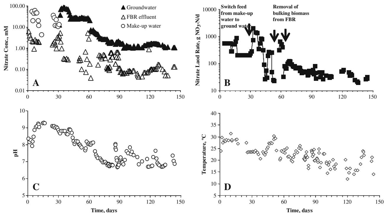
**Fig. 2** Operational performance of FBR. **a** Influent and effluent nitrate concentrations. **b** Nitrate loading rates. **c** Change of pH during operational period. **d** Change of temperature during operational period
