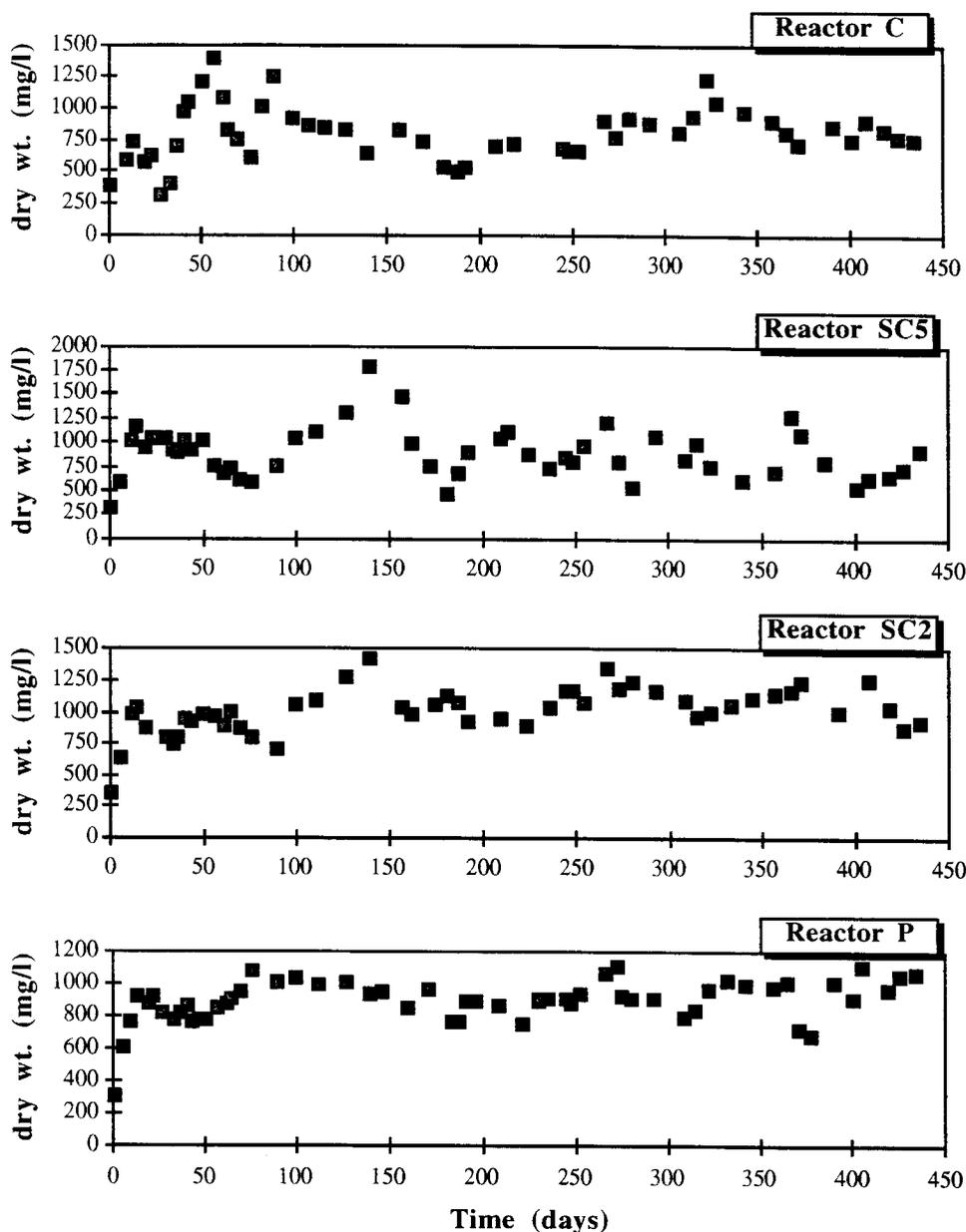
FIG. 3. Long-term variations in biomass concentration for each reactor enrichment community. Samples were taken at the end of the phenol addition period.
