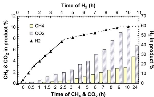
Fig. 2 – Gas concentrations in an MEC over a complete cycle (0.7 V applied voltage). The data show all gases produced during a cycle. (Nitrogen gas initially present in the reactor headspace is not included.)
