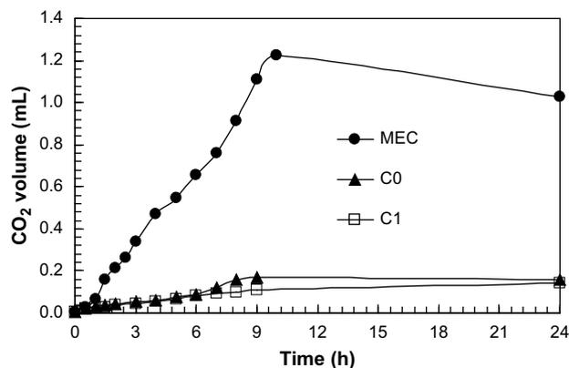
Fig. 4 – CO<sub>2</sub> production in the headspace of the MEC and control reactors.
