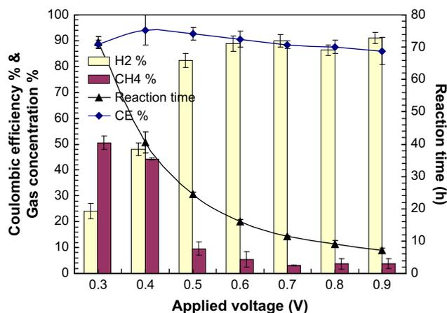
Fig. 6 – Coulombic efficiency, gas concentrations ( $H_2$  and  $CH_4$ ) and time needed for one full cycle as a function of different applied voltages.
