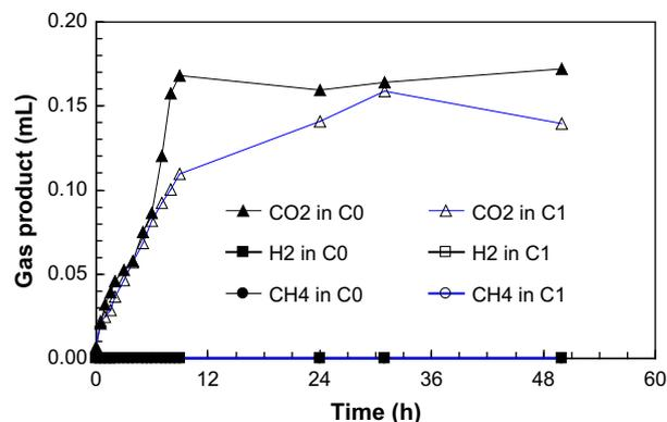
Fig. 3 – Gas concentrations in the headspace of the control reactors (open-circuit conditions).
