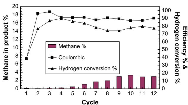
Fig. 1 – Methane production and hydrogen conversion efficiency in a single chamber MEC at 0.7 V applied voltage.
