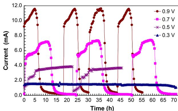
Fig. 7 – Current generation in MECs at different applied voltages showing changes in maximum current densities.
