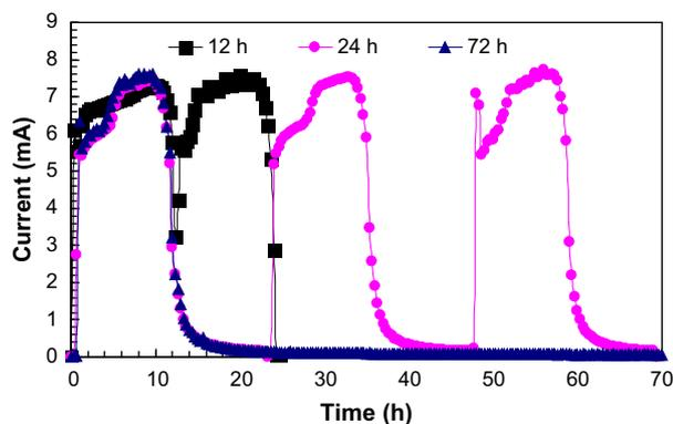
Fig. 5 – Effect of operation time on current generation in MECs over 70 h.
